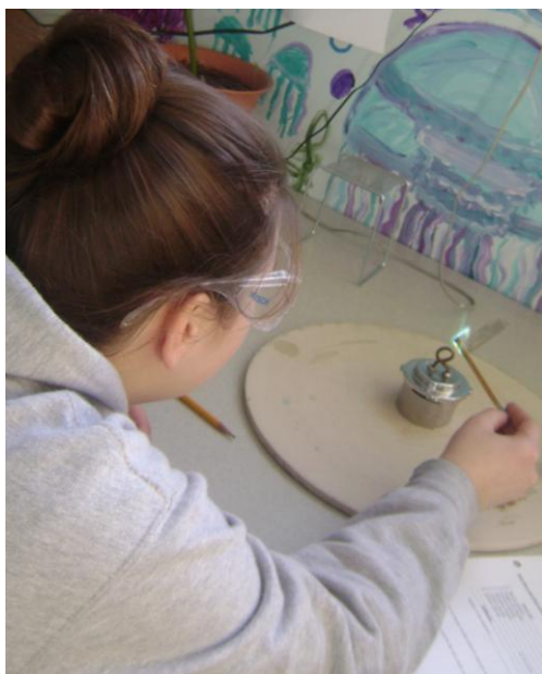
Lab to determine unknown metal ion based on unique characteristic color when burned
